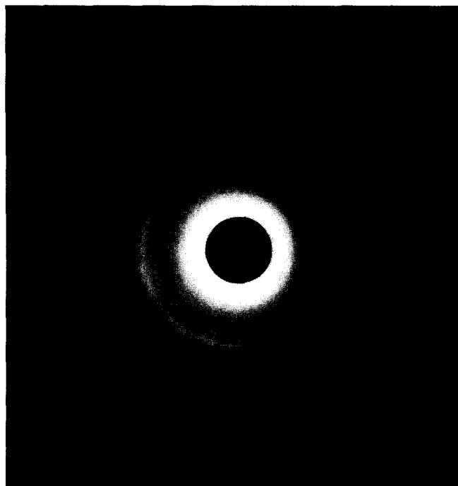
Figure 1 Typical X-ray diffraction pattern produced by polyether-sulphone containing dichloromethane
